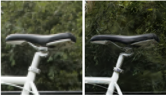
Figure 5: Left: Ground truth image of bike seat. Right: High frequency artifacts with 3DGS when sampling at higher rate.
